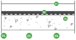
Concrete floating screed with 70 mm thickness
