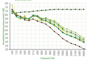
L<sub>nr</sub> - Normalized impact sound pressure level of the reference floor with the floor covering under test;  $L_{n,n}^{-}$  Normalized impact sound pressure level of the Lab reference floor;  $\Delta L_{n}^{-}$  Impact sound pressure level reduction index of the covering under test, on a normalized floor;
