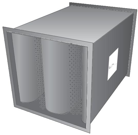
HLFL silencers provide improved low frequency attenuation with low pressure drop for higher velocity HVAC systems. The acoustic fill is totally encapsulated to prevent erosion or entrainment of particulate. A honeycomb acoustic stand-off provides additional protection and performance.
