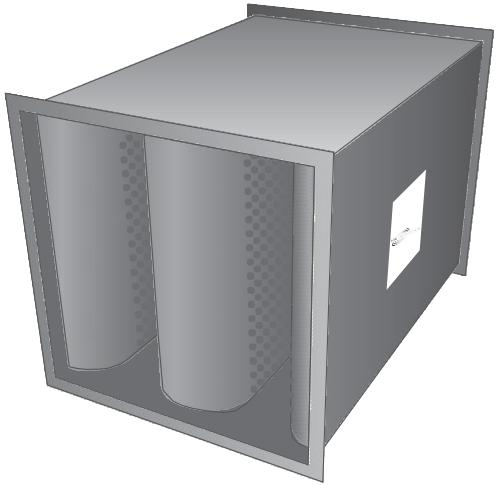
HLFM silencers provide improved low frequency attenuation for medium velocity HVAC systems. The acoustic fill is totally encapsulated to prevent erosion or entrainment of particulate. A honeycomb acoustic stand-off provides additional protection and performance.
