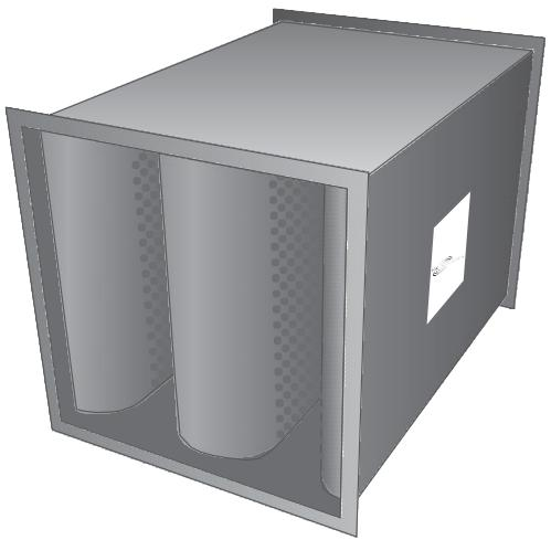
HLFS silencers are advantageous where low frequency DIL requirements are high in HVAC systems. The acoustic fill is totally encapsulated to prevent erosion or entrainment of particulate. A honeycomb acoustic stand-off provides additional protection and performance. Ideal for hospitals, laboratories and clean rooms.
