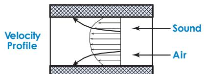
Reverse Flow occurs when air and sound waves travel in opposite directions, as in a typical return-air system. Under reverse flow conditions, sound is refracted away from the walls and towards the centre of the duct silencer.
